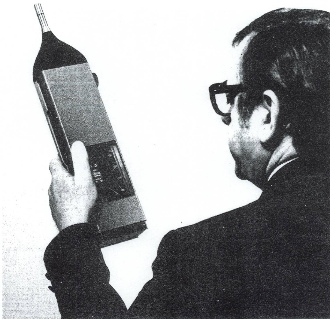
Figure 1-13. Random Response Microphone in Use
